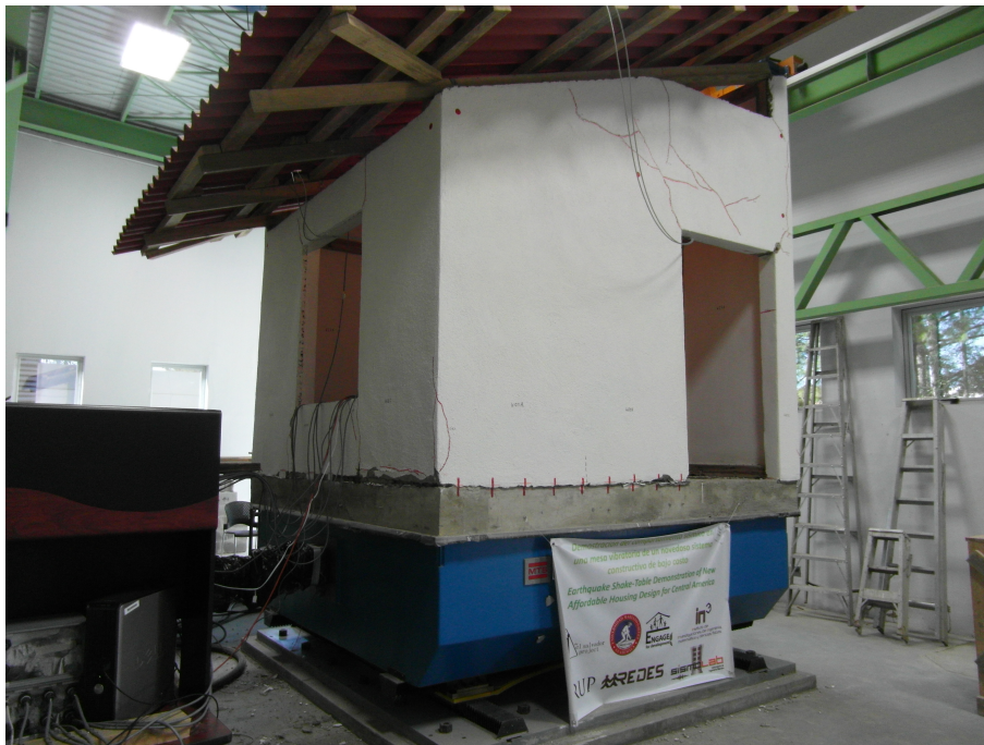
Figure 10. Damage state at end of bi-directional shake-table testing for a full-scale model of a room of a house at the Universidad Mariano Gálvez in Guatemala City (Kaminski, 2015)
