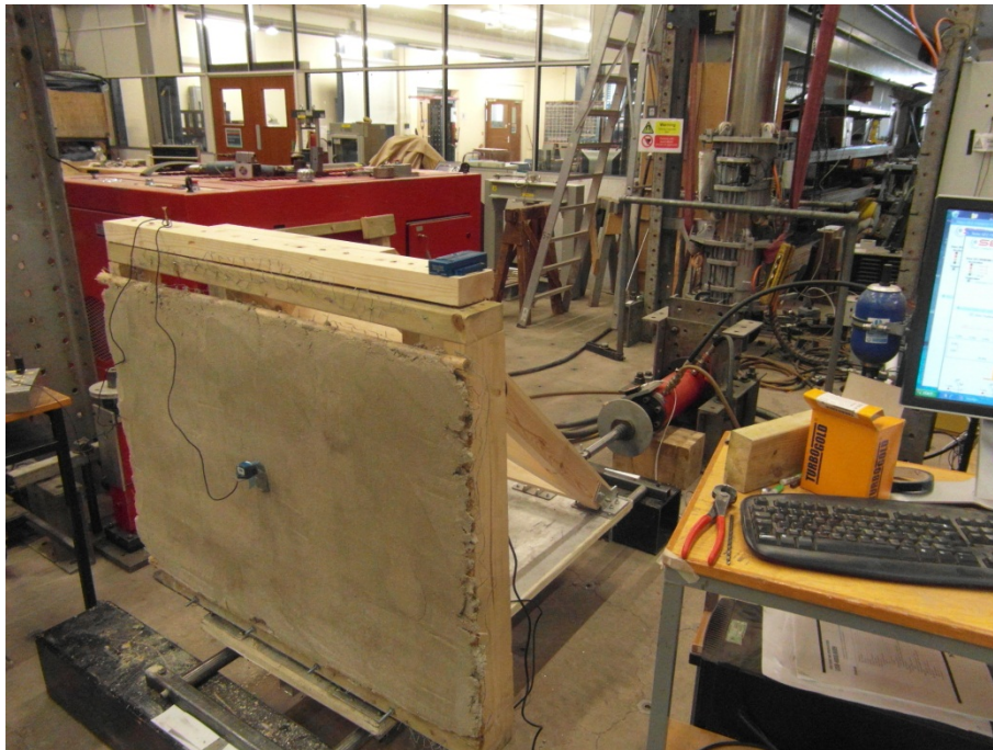
Figure 9. Out-of-plane testing of wall panels on a uni-directional shake-table at Cambridge University (Kaminski, 2015)
