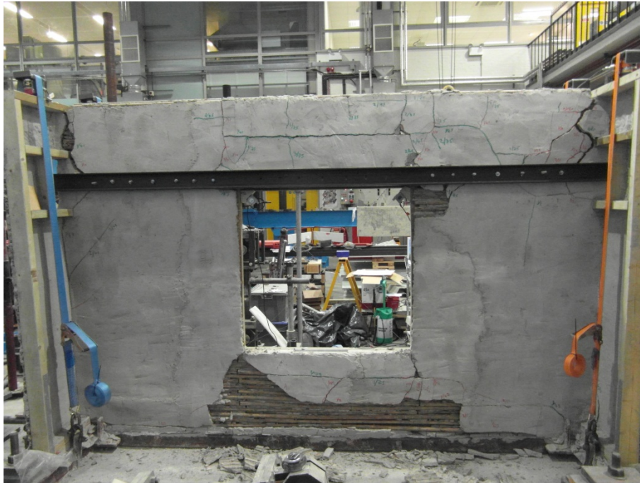
Figure 8. In-plane testing of wall panel at Imperial College London, 2013. Image shows typical damage state at failure, using singly-sided chicken mesh on reverse side only (Kaminski, 2015)
